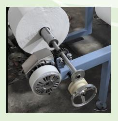
The gauze material roll tension controlled by magnetic powder clutch, machine running with stable tension.
