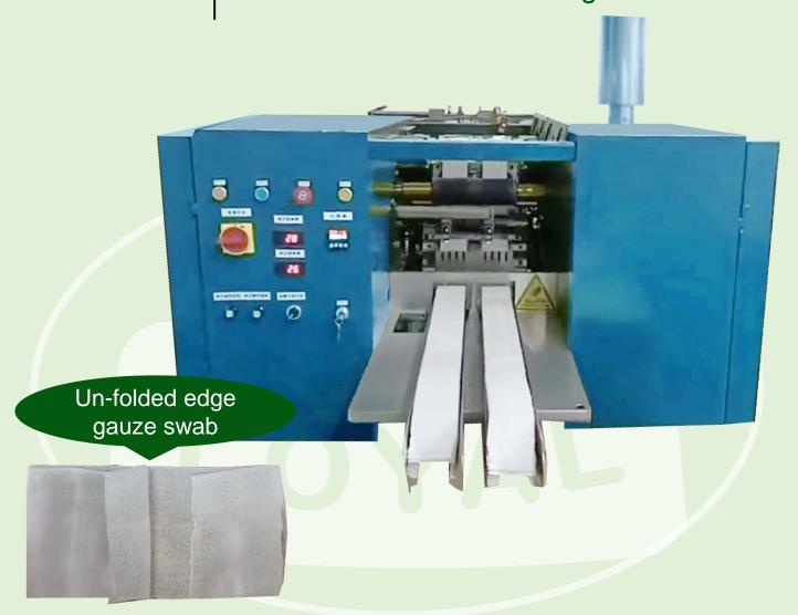
Series high speed gauze swab folding machine can meet most of the standard gauze swab folding methods, such like folded edge or un-folded edge, 5x5cm, 7.5x7.5, 10x10cm, 8ply, 12ply, 16ply.
