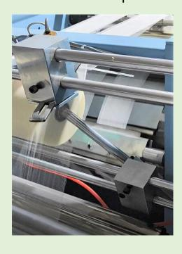
Via simple adjustment, different tier (4ply, 8ply, 12ply and 16ply) can be done in ONE machine.
