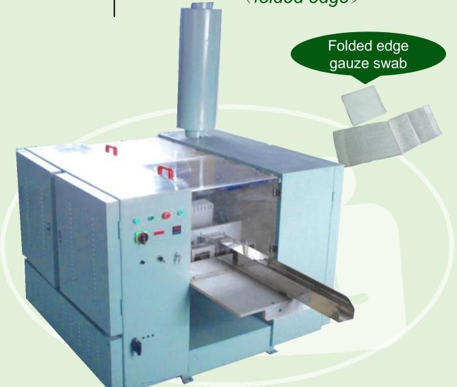
Series high speed gauze swab folding machine can meet most of the standard gauze swab folding methods, such like folded edge or un-folded edge, 5x5cm, 7.5x7.5, 10x10cm, 8ply, 12ply, 16ply.
