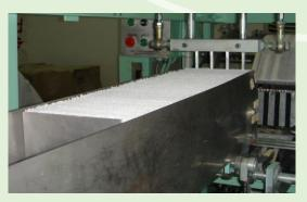
The output tracks from 1-6 lanes which will customized according gauze swab folding method and size request.
