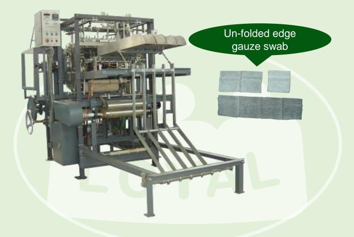
Series gauze swab folding machine can do customize to meet most of the gauze swab folding methods, sizes and tier request, such like folded edge or un-folded edge, with or without X-ray thread, 5x5cm, 7.5x7.5, 10x10cm, 8x18cm, 7.5x10cm,10x20cm, 4ply, 8ply, 12ply, 16ply, etc.
