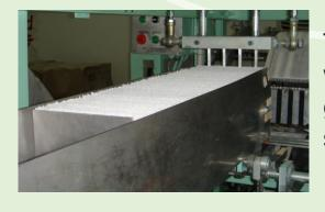
The output tracks from 1-6 lanes which will customized according gauze swab folding method and size request.
