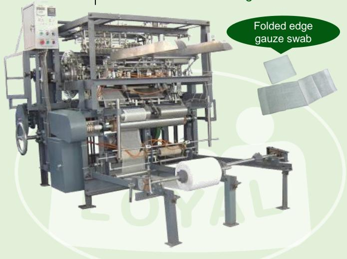
Series gauze swab folding machine can do customize to meet most of the gauze swab folding methods, sizes and plies request, such like folded edge or un-folded edge, with or without X-ray thread, 5x5cm, 7.5x7.5, 10x10cm, 8x18cm, 7.5x10cm,10x20cm, 4ply, 8ply, 12ply, 16ply, etc.
