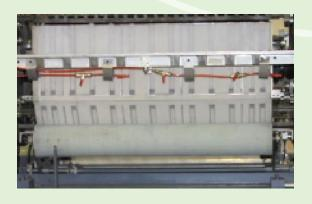
Key part--cuter, it is made by alloy tool steel, available to use in a long service life.
