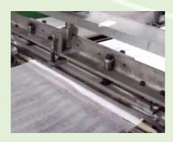
Key part--cuter, it is made by alloy tool steel, available to use in a long service life.
