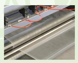
During winding, the tension control device works to make it suitable to cut raw gauze with too many joints and unbalanced tension.
