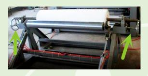
The raw material holder has regulating function which can adjust the position of gauze jumbo roll position within range of +2.5cm.
