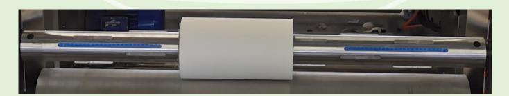
The re-winding rolls are adopt air shafts, which can easily adjust tension and fast remove and remount.
