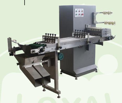
Rubbing various diameters of cotton slivers to fixed weight and diameter of cotton balls.
