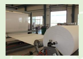
The automatic tension control system responses sensitively, responds fast, be qualified for different gram weight of spunlace non-woven fabric, maximum guarantee spunlace (very sensitive tension) non-woven not been deformation during the slitting and rewinding process.
