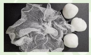
Automatically unwind the gauze (or non-woven) material roll, cutting the fabric at fixed size, feeding the rubber pipe and cut the pipe as an small size elastic rubber ring. The folding system will make the gauze (or non-woven) material incorporate into the rubber elastic ring, following series of folding and winding steps, a gauze (or non-woven) ball been making done.
