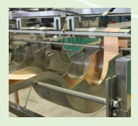
Active unwinding system and prefeeding system ensure the bandage winding tension stable, bandage will not been elongation during winding process spin speed variation.
