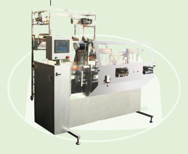
Automatically unwinding the materials rolls, feeding, winding, length counting, cutting and output the bandage.
