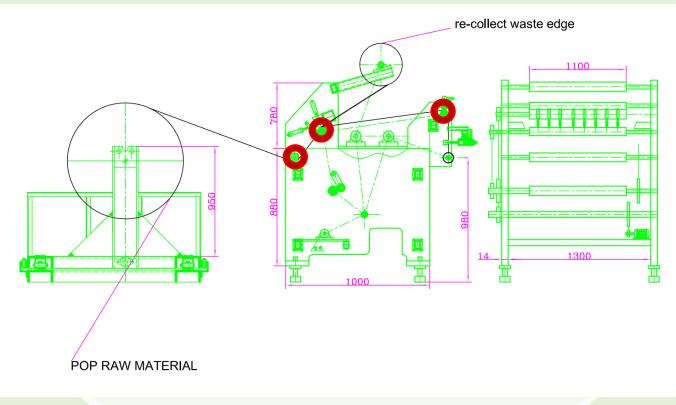
From unwinding jumbo material roll to small bandage rolls, the fabric only through three shafts (red ring in above drawing), powder drop rate is much reduced compare with traditional slitting machine.
