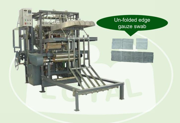
Series gauze swab folding machine can do customize to meet most of the gauze swab folding methods, sizes and tier request, such like folded edge or un-folded edge, with or without X-ray thread, 5x5cm, 7.5x7.5, 10x10cm, 8x18cm, 7.5x10cm, 10x20cm, 4ply, 8ply, 12ply, 16ply, etc.
