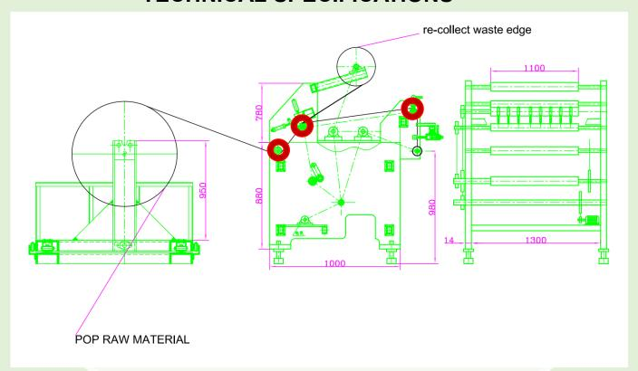
From unwinding jumbo material roll to small bandage rolls, the fabric only through three shafts (red ring in above drawing), powder drop rate is much reduced compare with traditional slitting machine.
