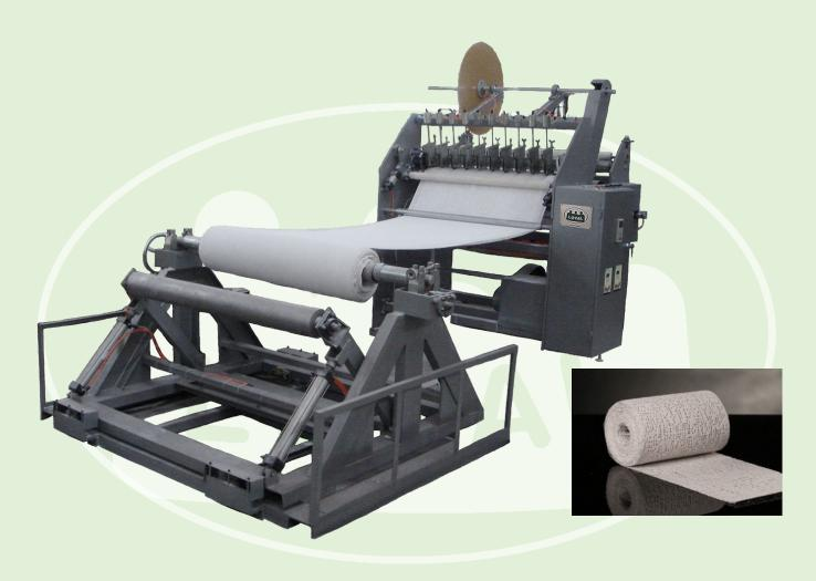
Automatically unwinding, deviation correction, slitting, length counting, re-winding, auxiliary demount.
